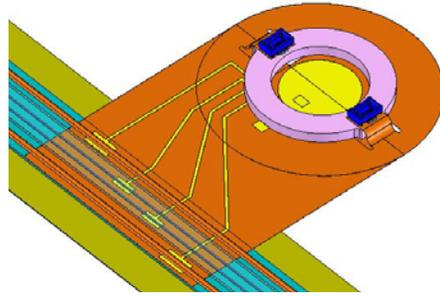
Figure 3: Schematic of SHM node flexible circuit w/tail
