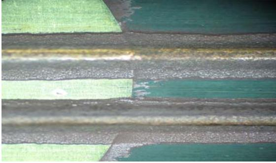
Figure 4: Shorted traces due to melted PFS powder
