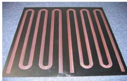
Figure 5: Meandering PFS traces on a CFRP plate
