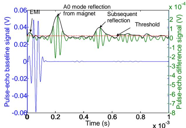
Figure 9: Pulse-echo with magnet in near position
