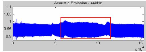
Figure 4: Air pump acoustic emission with faults introduced
