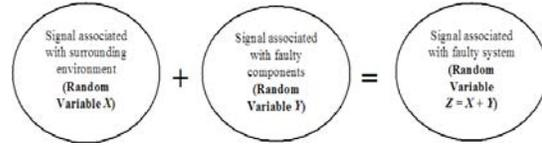
Figure 3: Linear combination of random signals associated with surrounding environment and faulty components
