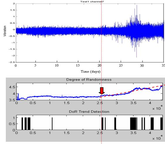
Figure 12: Early detection using sensor #4 in  $x$ -direction
