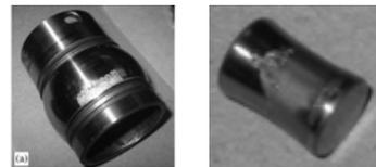
Figure 9: Defects in bearings #3 (left) and #4 (right) given in (Qiu, 2006)
