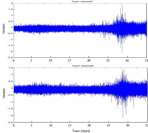
Figure 10: Vibration data of sensor #4 in  $x$ -direction (top) and  $y$ -direction (bottom)
