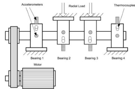
Figure 8: Experimental system setup
