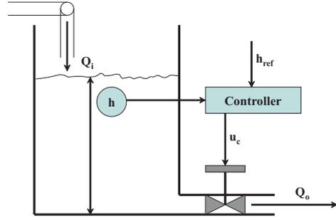
Figure 1: Our system is made up of tank, a valve and one controller.
