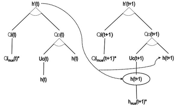
Figure 2: Possible conflict for the tank system with integral approach. A discrepancy can be found between  $h(t+1)$  estimation and  $\hat{h}_{obs}(t+1)$  (the discrepancy node is graphically represented by a ellipse). If there is no discrepancy,  $h(t+1)$  is used for next simulation period.
