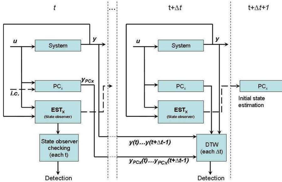
Figure 5: Integration scheme: estimation given by state observers,  $EST_x$ , can be used directly for fault detection, or can be used as initial states estimation for the next simulation period in the same MEM implemented as a simulator,  $PC_x$ .
