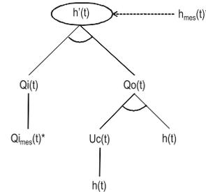
Figure 3: Possible conflict for the tank system with derivative approach. A discrepancy can be found for  $\dot{h}(t)$  using measurement of level  $LT1$ ,  $h_{mes}$ , or direct estimation of the derivative from previous values for  $LT1$  (the discrepancy node is graphically represented by an ellipse).
