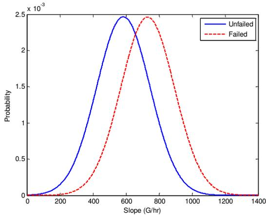
Figure 5. Fitted statistical distributions of unfailed (blue) and failed (red) slopes of the cumulative stress path.
