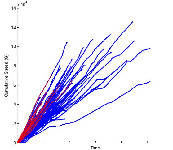
Figure 4. Cumulative stress paths for unfailed (blue) and failed (red) tools.
