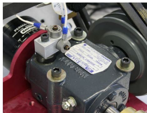
Figure 4. The gearbox with installed accelerometers.
