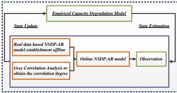
Figure 2. Fusion-data-model Framework for Lithium-ion Battery RUL Estimation
