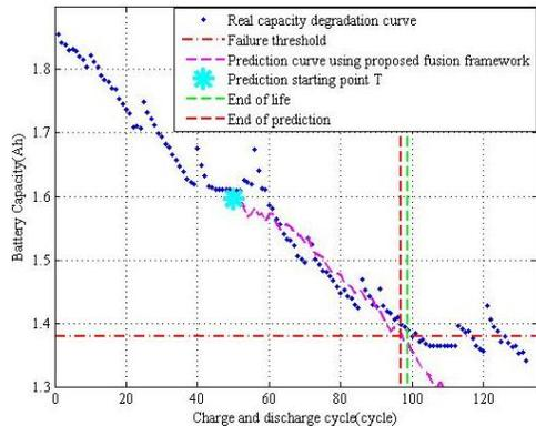
Figure 4. RUL prediction based on proposed fusion framework for NASA Battery #18 (Form 2)
