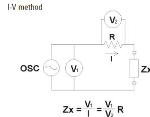
Figure 1. Basic circuit for impedance measurement
