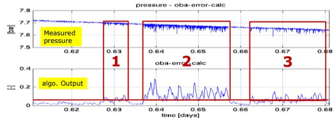
Figure 14. Top graph, measured pressure signal. Bottom graph, output of connection defects detection algorithm
