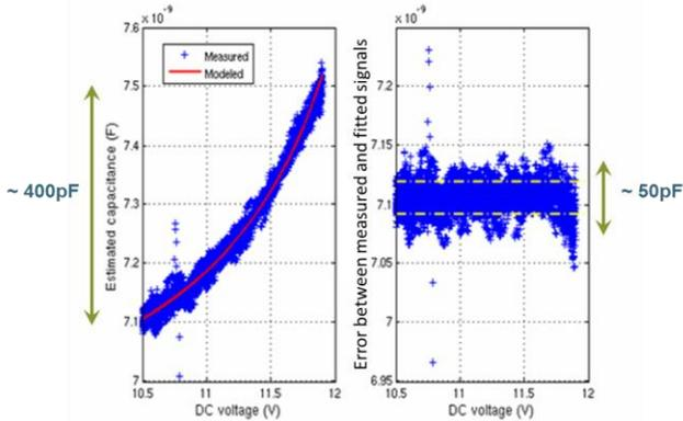
Figure 12. Compensation for equivalent impedance variation due to PWM voltage (left graph: non-compensated capacitance estimate, right graph: compensated capacitance)
