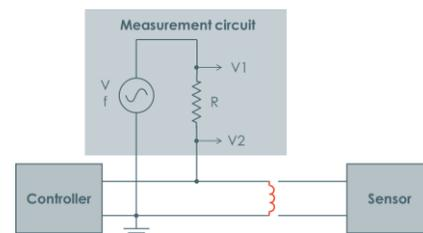
Figure 2b. Impedance measurement circuit used to diagnose short connection fault in an industrial circuit. R should be small.
