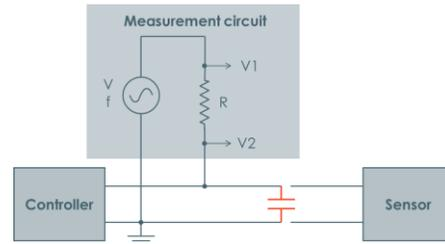
Figure 2a. Impedance measurement circuit used to diagnose open connection fault in an industrial circuit. R should be large.
