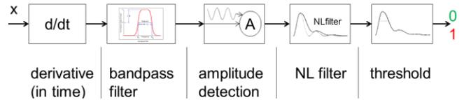
Figure 6. Block diagram of the connection fault detection algorithm
