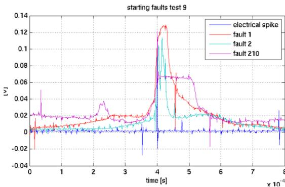
Figure 5. captured voltage for different connection faults during a test
