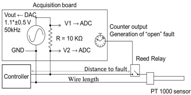
Figure 8. validation set-up for impedance measurement with a resistive load
