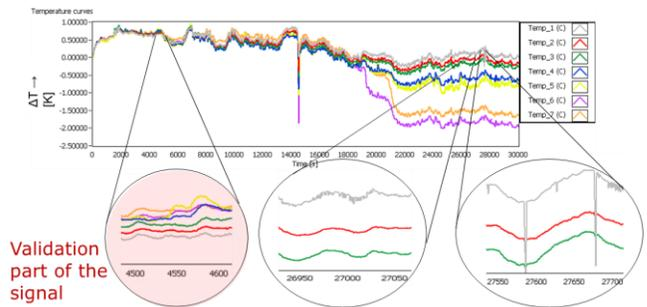
Figure 15. Measured temperature signals from an industrial application where one of the measured signals contain connection faults
