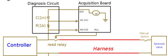
Figure 11. validation set-up for impedance measurement with a complex load
