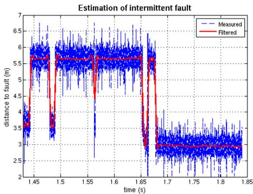
Figure 9. estimation of distance to fault for an intermittent open connection fault
