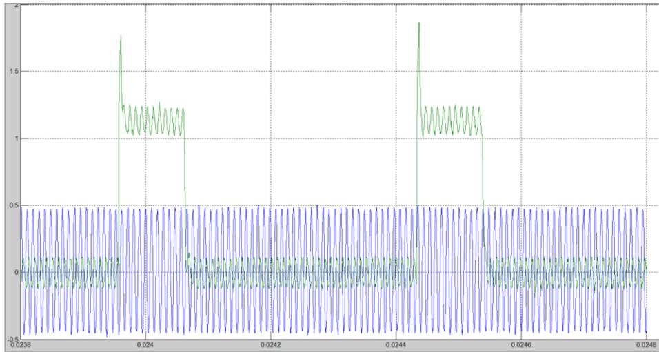
Figure 3. Captured voltages  $V_2$  (green) and  $V_1$  (blue) (as described in figure 2a and 2b) when using a resistive sensor
