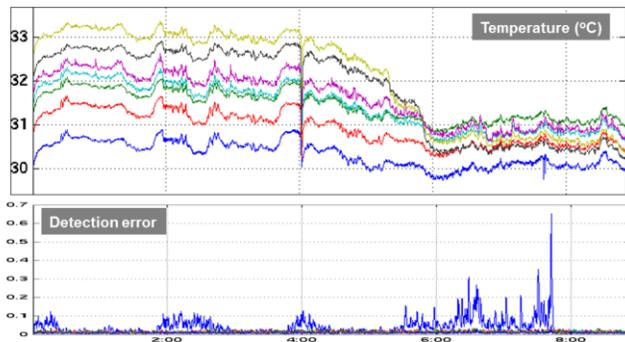
Figure 16. Detected connection fault in one of the temperature signals
