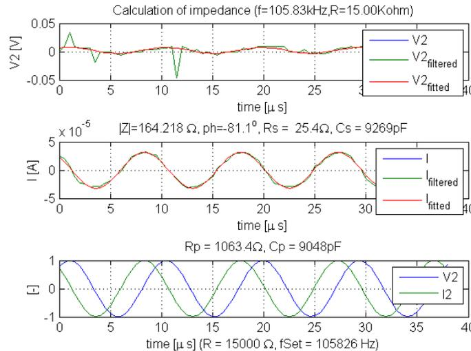
Figure 4. curve fitting and equivalent impedance estimation ( $|Z|$ : equivalent estimated absolute impedance,  $ph$ : estimated phase between current and voltage,  $R_s$ ,  $C_s$ : Equivalent series resistance and capacitance),  $R_p$ ,  $C_p$ : equivalent parallel resistance and capacitance)
