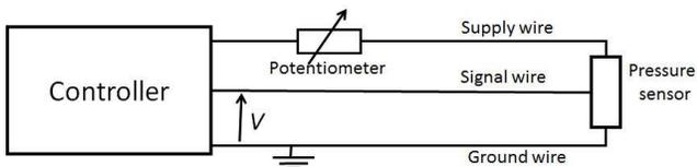
Figure 13. Set-up for connection faults generation in the supply wire of a pressure sensor.
