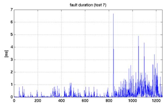
Figure 7. Connection faults duration on 20 hours accelerated lifetime testing of industrial connectors.
