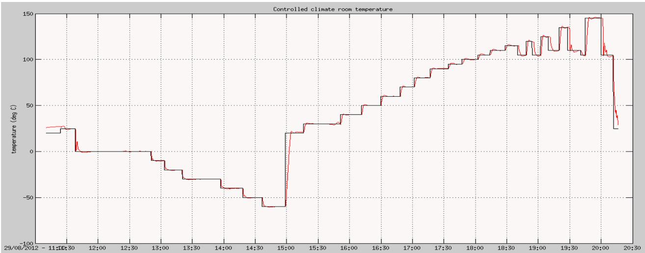
Figure 8. Step stress to identify thermal stress limits (black line: set temperature, red line: measured temperature)
