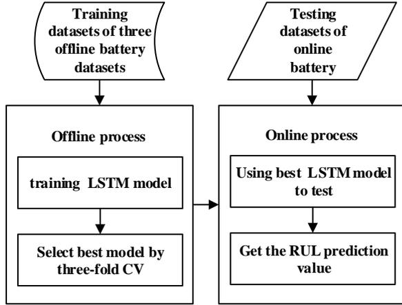
Figure 3. The lithium-ion battery RUL prediction diagram using LSTM.
