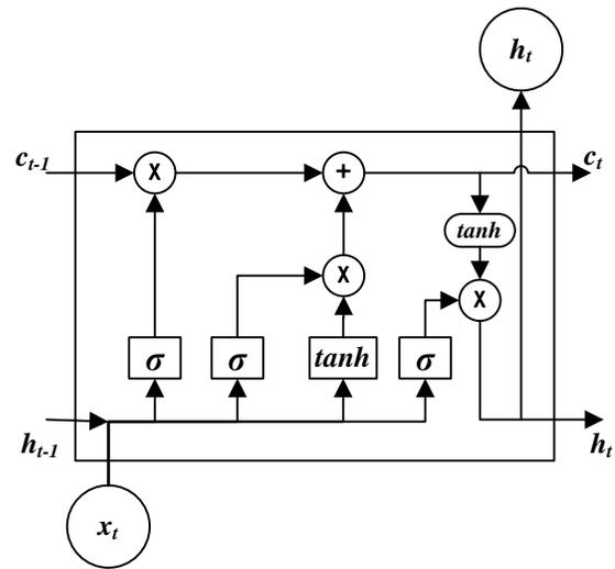
Figure 2. The diagram of LSTM.
