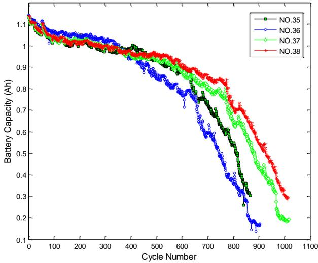
Figure 4. The capacity degradation curves of #35, #36, #37 and #38 batteries.
