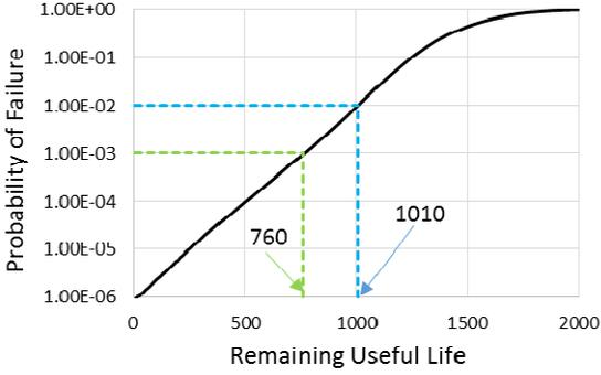
Figure 6. The Probability of Failure of Remaining Useful Life for Measurement Set in Figure 2 Case 1
