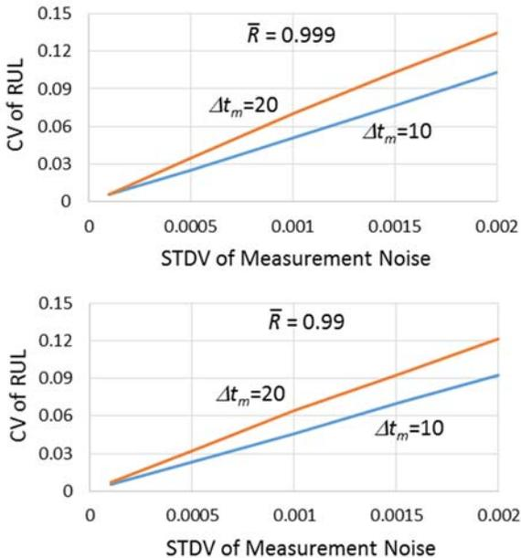
Figure 7. CV (Coefficient of Variation) of RUL vs STDV of Measurement Noise
