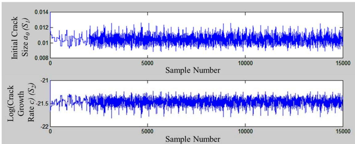
Figure 3. Samples of Crack Size  $a_0$  and Log of Crack Growth Rate  $c$  for Measurement Set of Case 1 in Figure 2
