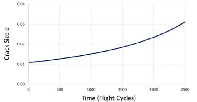
Figure 1. Ground Truth Crack Growth Curve for Case Study
