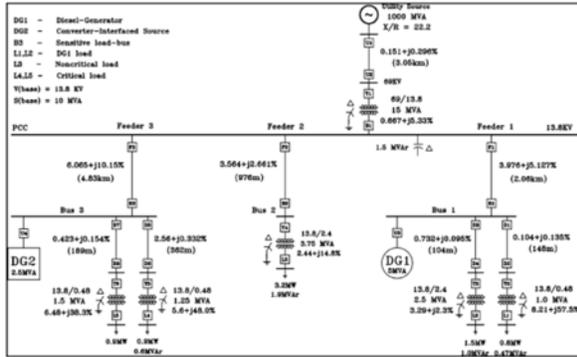
Fig.1. Single-line diagram of the study system [10]
