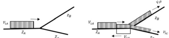
Fig. Traveling wave of voltage encountering a line bifurcation
