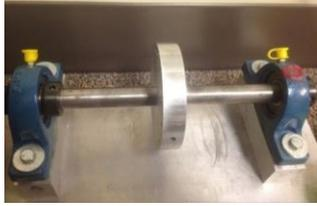
Figure 3. Rotor shaft test bed
