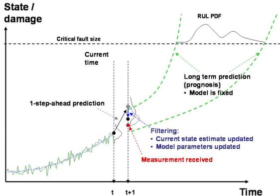
Figure 1: Concept of process model-based prognostics.
