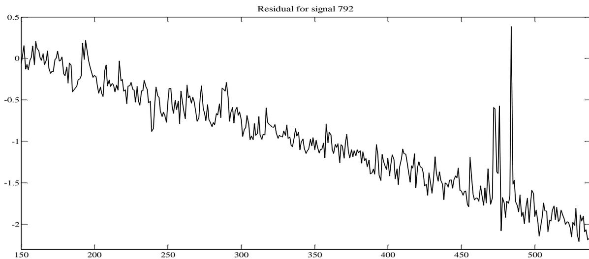
Figure 3: Residual computed for signal 792
