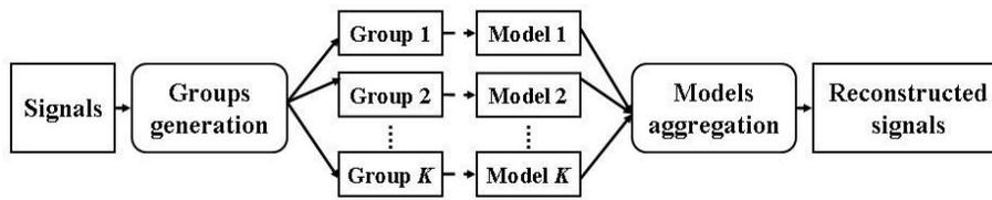
Figure 1: The ensemble approach to large-scale signal reconstruction
