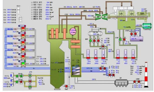
Fig. 2. An example of DCS screen for 250MW coal-fired power plant.
