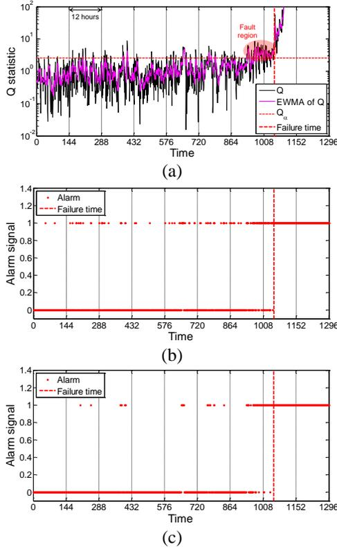
Fig. 7. (a) Q statistics and EWMA for the test samples on a semi-logarithmic scale (b) alarm signal without EWMA (c) alarm signal with EWMA.
