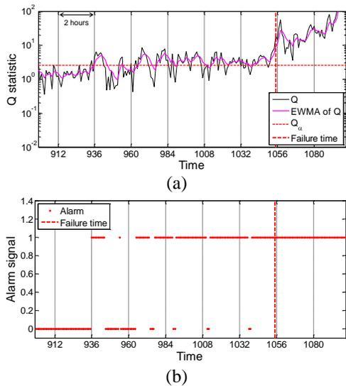
Fig. 8. Enlargement of failure symptom region in Fig. 7 (a): (a) Q statistic and EWMA; (b) alarm signal with EWMA.
