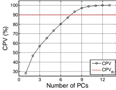
Fig. 5. Results of the CPV method for determining the retained number of PCs.
