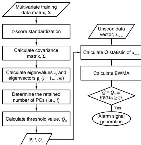
Fig. 1. PCA-based fault detection procedures.
