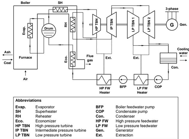
Fig. 3. Simplified schematic diagram of the coal-fired power plant.
