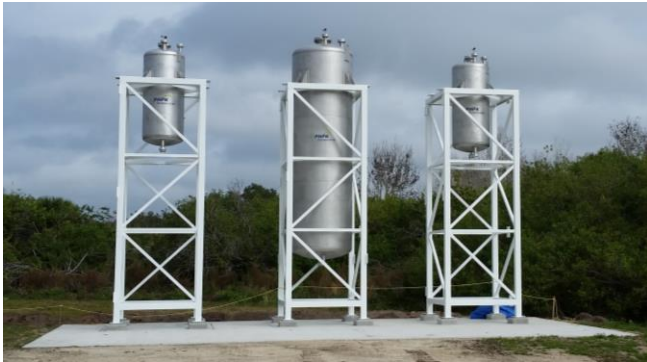
Figure 5. LO2 DTS Vehicle Simulator
