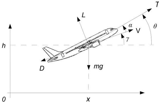
Figure 1. The aircraft forces and angles during vertical flight with nonzero climb rate.
