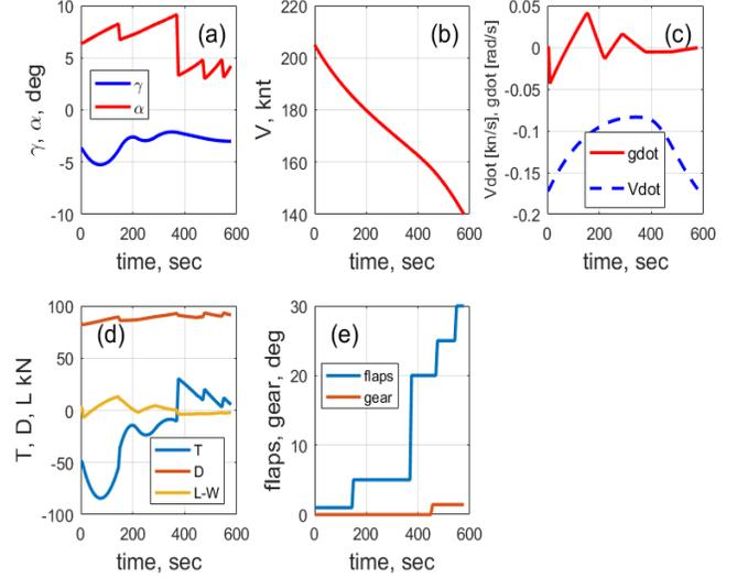
Figure 4. Aircraft dynamics reconstructed from the flight profile defined as  $h(x)$  and  $V(x)$ : (a)  $\alpha(t)$  and  $\gamma(t)$ ; (b)  $V(t)$ ; (c)  $\dot{\gamma}(t)$  and  $\dot{V}(t)$  (d)  $T(t)$  - thrust,  $D(t)$  - drag, and  $L(t) - W$  - lift minus weight; (e) flaps and landing gear configuration.
