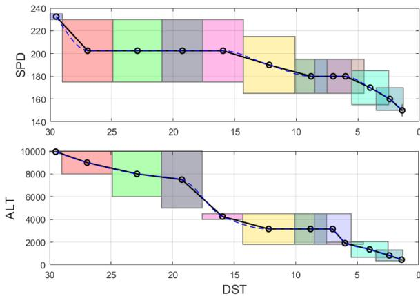
Figure 3. Vertical flight profile obtained by interpolation of the phase transition points: linear interpolation (solid black lines); cubic interpolation (dashed blue lines). Color shaded boxes show bounds on the speed, altitude, and distance introduced in the Table 1.
