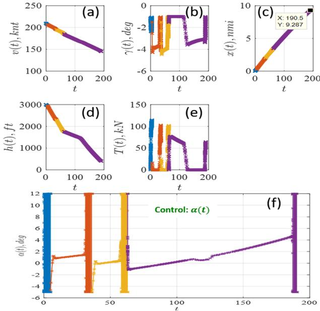
Figure 2. Minimization of transition times for descending trajectory with 4 phases. The figures show the dependence of dynamical variables of the system on time: (a) Velocity; (b)  $\gamma$ ; (c) distance; (d) Altitude; (e) Thrust; and (f) Angle of attack. Different colors indicate different phases of the flight and correspond (left to right) to phases (i) to (iv).
